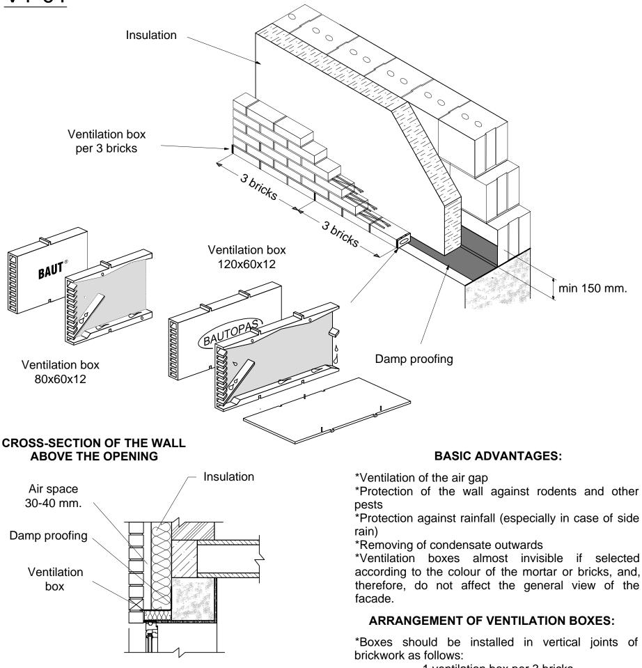
1 ventilation box per 3 bricks <sup>\*</sup>2 rows of boxes in the building of up to two floors (at the bottom - within the first row of brickwork and at the top – within the last one)
